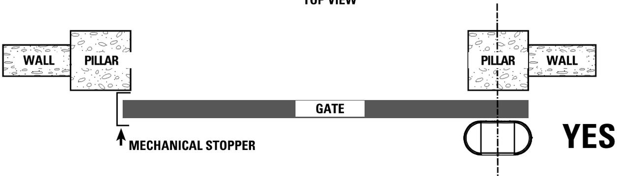
Engine support plate must be fixed at 5 cm from the gate :
