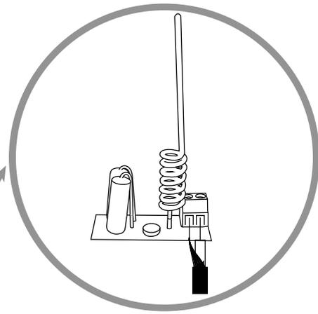
If you want to improve the operating range of your remote, you can connect the blinker antenna with a RG58 coaxial cable (not supplied). In this case you must disconnect the original antenna and then connect the coaxial copper core to the terminal ANT and the coaxial braided shield to the terminal GND on both antenna and electronic card.
