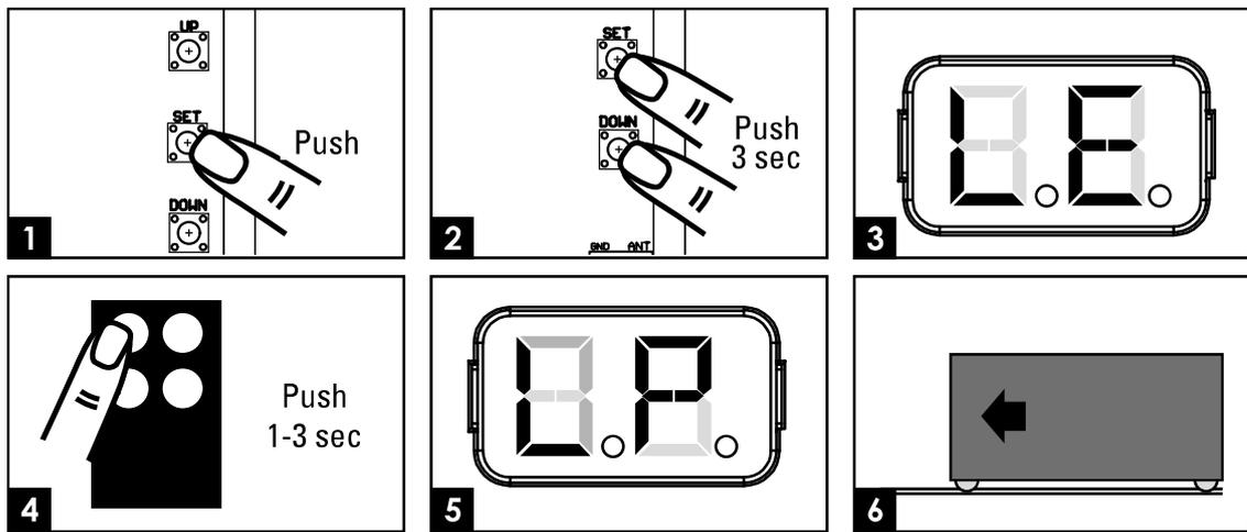
If your gate is opening when you start the programming, stop the program to push on SET. L» appears on the display, wait for it to turn off then go on the program 1 to reverse the rotation direction of your gate (see following page).
