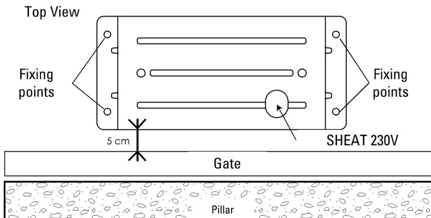
Drill your concrete substrate and install your 4 metal or chemical anchors dowels to secure your engine support plate.
