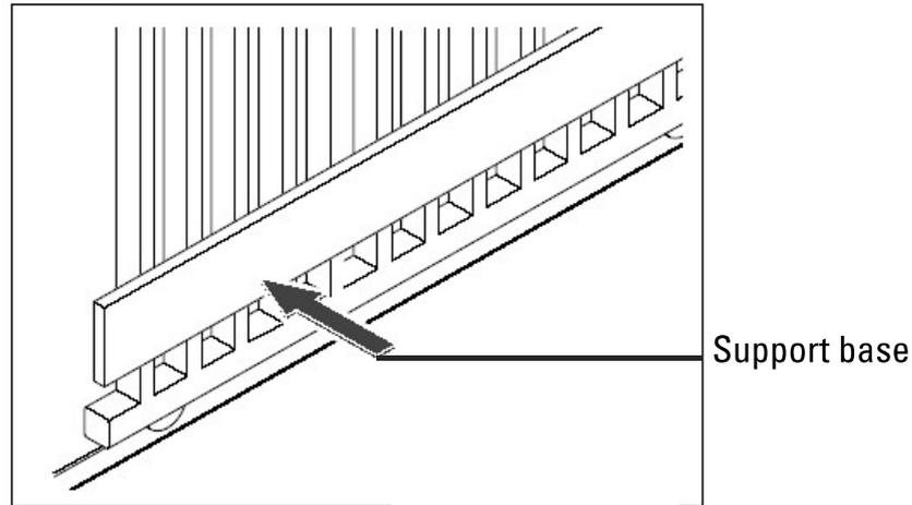
To place the first rack, put it down respecting a 2 mm space between the engine's toothed wheel and the rack as indicated on the scheme below :
