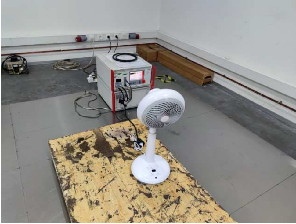
Photograph 6: Set-up for immunity test of injected current
