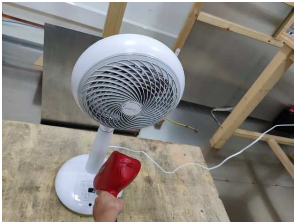
Photograph 4: Set-up for immunity test of radio frequency electromagnetic field
