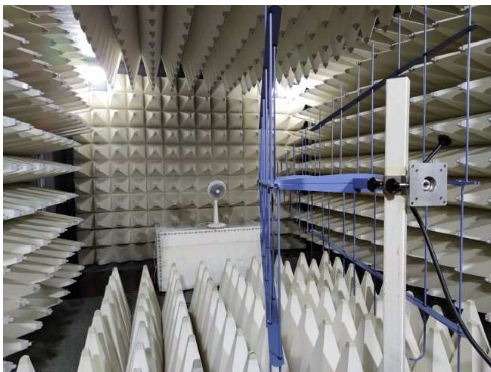
Photograph 4: Set-up for immunity test of radio frequency electromagnetic field
