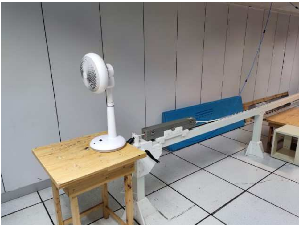
Photograph 2: Set-up for measurement of disturbance power
