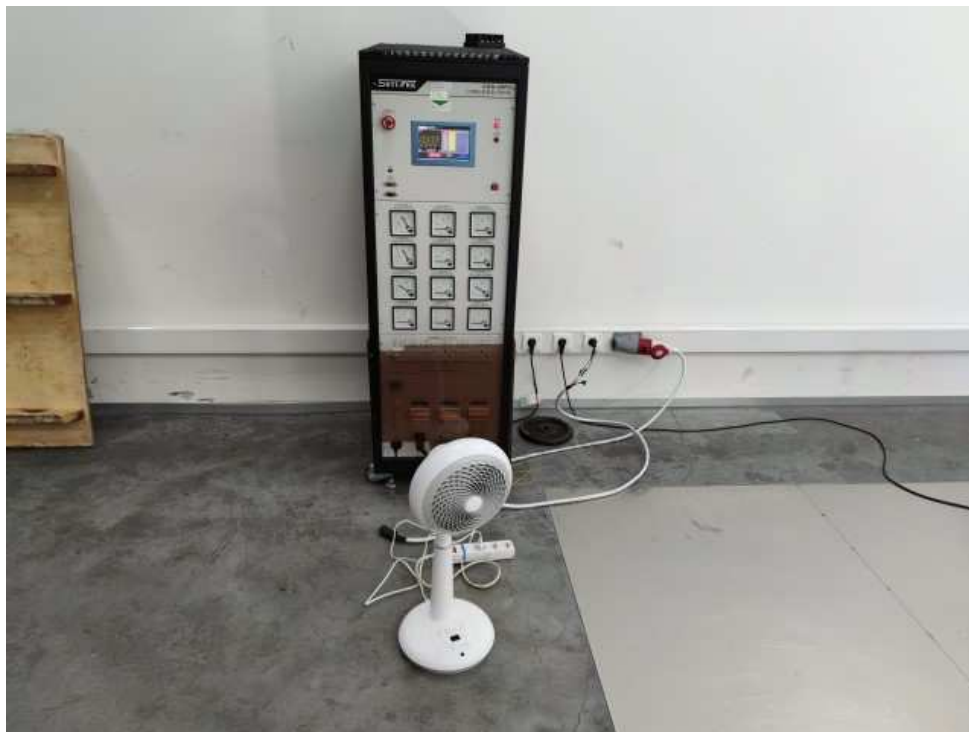
Photograph 7: Set-up for immunity test of voltage dips
