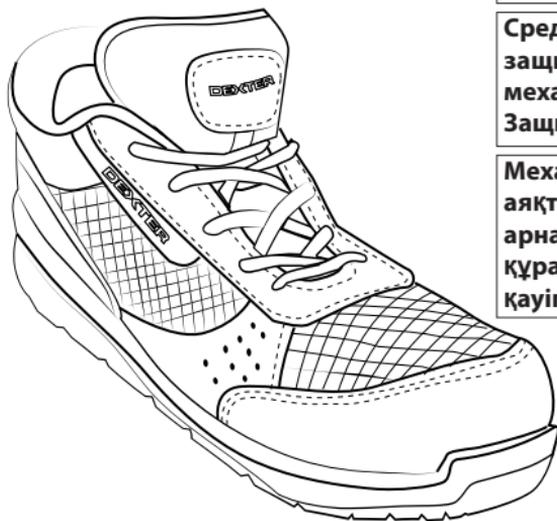
Means of individual protection of feet (shoes) from mechanical influences. Protective footwear S1 P SRC.
