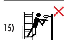
15) Do not impose a side loading, e.g. when drilling into masonry and concrete.
