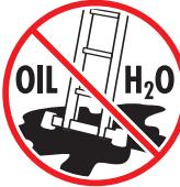
It is prohibited to place the ladder on slippery surfaces, eg ice, polished surfaces or on visibly soiled solid surfaces if additional measures have not been taken to prevent the ladder from slipping and to guarantee sufficient cleanliness of the site.
