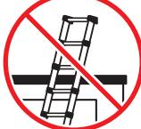
ALWAYS position the ladder on the upper support and under no circumstances using the rails or rungs, which could thereby be damaged.
