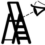
Visually inspect the ladder for damage to ensure that it is safe to use at the start of each working day that the ladder will be needed.
