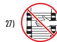
27) Pay attention to the position and placement of the hands when the telescopic ladder is again being collapsed.
