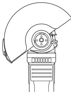
Please use grinding protective cover for grinding operation.
